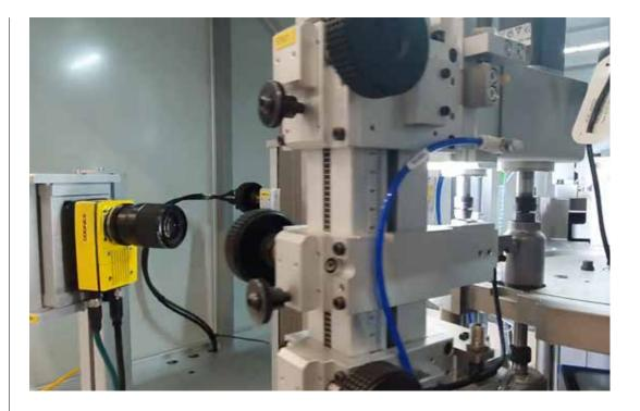
The linear camera, combined with an encoded 360° rotation station, allows you to reconstruct the image of the lateral development of pieces with cylindrical or similar geometry.
