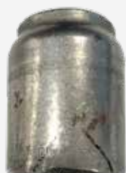
Missing Material on the Skirt/Head Missing Head
