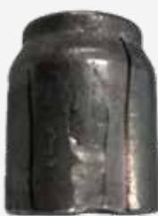
Missing Material on the Skirt/Head Missing Head
