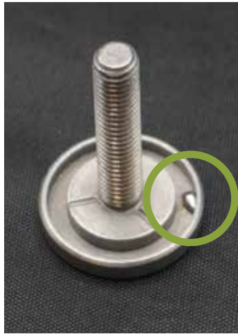
DEFECT ON INNER SIDE OF THE FLANGE
