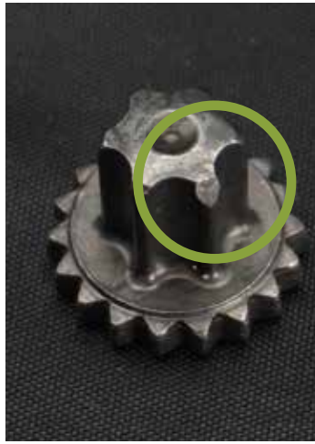
SIDE DEFECT ON PINION
