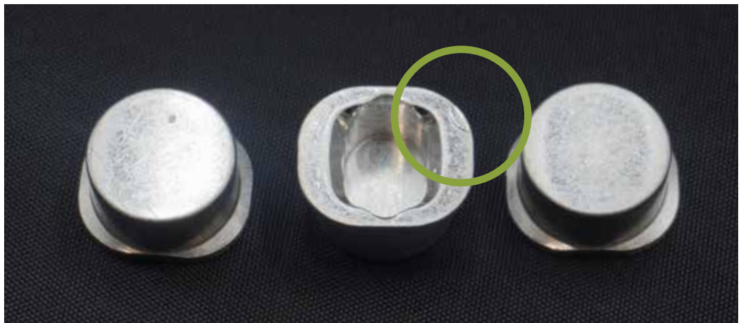
MOLDING DEFECT ON CAR PARKING SENSOR CAPS
