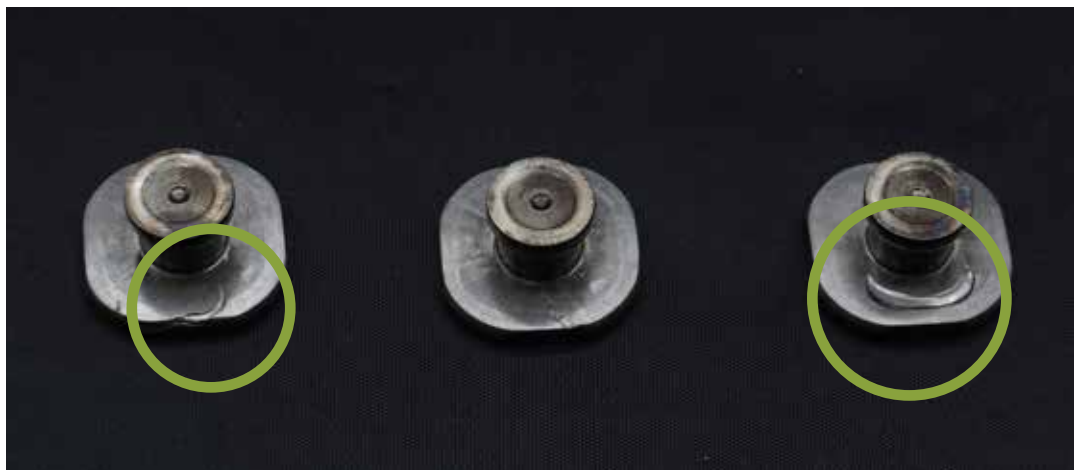
MOLDING DEFECT ON METAL PARTS
